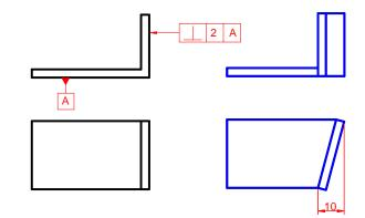
Fig. 4. After processing, the tilted top surface was observed. Does the product comply with the specification?
