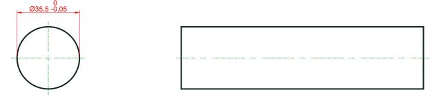
Fig. 11. A digital calliper 0-150 mm with a resolution of 0.01 mm was used for the diameter measurement of the shaft shown in the figure above. The result was 35.48 mm. Does the product comply with the specification?
