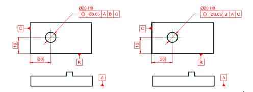
Fig. 10. Are these two specifications equivalent?
